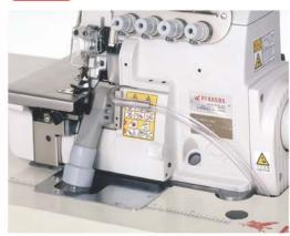
This pneumatic device strongly sucks up cutting waste and fine dust generated during sewing, providing clean and comfortable working conditions.
