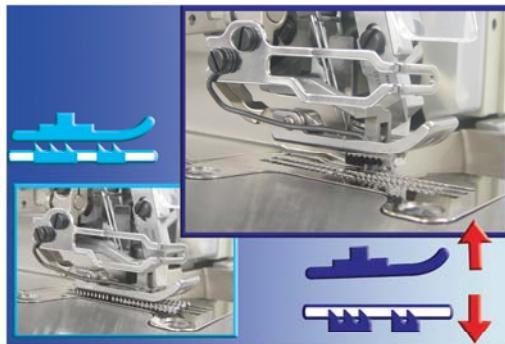
Since a drop feed mechanism is employed, the bottom feed dogs drop below the top surface of the needle plate when the presser foot is raised. Use of this mechanism enables smooth fabric loading.
