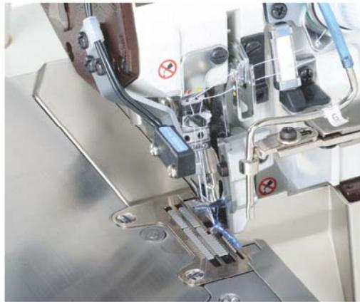
The thread chain is automatically sewn into the overlock seams at the start of sewing. Thanks to this feature, this machine prevents the seams from unraveling, reducing one bartacking operation, and dramatically increasing productivity.
