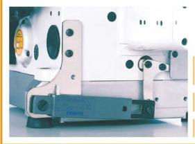
Thanks to this device, no unraveling occurs because the stitches become automatically finer at the end of sewing. The need for a subsequent anti-unraveling operation is eliminated and quality of sewn products is increased.
