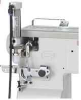
Pressing the treadle with your heel raises the presser foot. This device is easy to use, thus decreasing operator's fatigue and increasing productivity.
