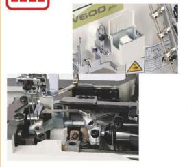
This device reliably reduces heat generated at the point of the needle by friction when they penetrate the fabric with the machine running at high speed. In addition, it allows the thread to move smoothly through the machine, decreasing the cause of stitch skipping and/or thread breakage. As a result, the machine produces uniform stitches.
