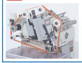
Thanks to the top feed belt, the top ply of material is fed positively, making this device suitable for plain seaming operations on particularly slippery fabrics such as nylon taffeta and quilting ,etc.lt is very effective for operations on knitwear where plyshift is a problem such as piping on training wear etc.
