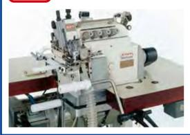
This device holds the fabric and elastic for the sewing of tubular goods, such as attaching elastic to waists. Thanks to this device, finished products are uniform, regardless of the operators skill.
