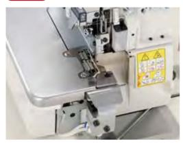
Thanks to this device, the thread chain is backlatched by sewing it into the overlock seams at the start of sewing in a sleeve closing operation and other similar operations. This feature prevents the threads from unraveling at the start of sewing and then eliminates the need for bartacking.
