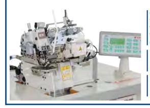
Conventionally, this operation requires a high level of techniques. However, the elastic feeder/inserter with tape/thread chain cutter (MC) deskills the operation because it feeds the proper amount of elastic according to the machine speed and the automatic tape/thread chain cutter cuts the elastic based on preset data. Thanks to this device, attaching elastic accurately and uniformly to tubular goods is easy.
