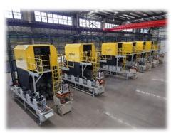
Factory facilities include the installation of environmentally friendly aluminum melting and holding furnaces fitted with individual smoke collectors
