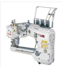
wide knife, the amount of the fabric is fed progressively as each stitch is being sewn, so this feature prevents the fabric from pushing back when the fabric is cut. This reduces sewing defects and presents a beautiful end product.
