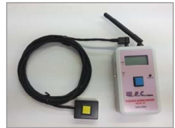
Left: Extension switch cord Right: Wireless switch
