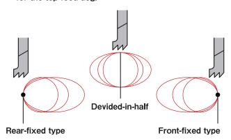
The amount of the top feed dog up-and-down movement is widely adjustable, from 2.6 mm to 5.0 mm (standard: 4.0 mm).
