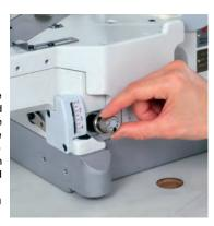
Easy-to-adjust differential feed ratio with the lever (available for an intermittent adjustment)
