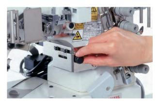
The amount of the top feed dog front-to-back movement is adjustable up to 6 mm (standard: 1.0 mm - 4.0 mm).
