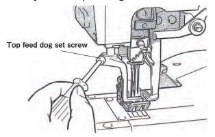
A diamond cut is employed for the top feed dog, in order to feed the fabric more smoothly and efficiently.
