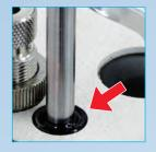
New type of oil-seal in the top of needle bar bushing.
