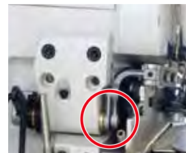
<Presser arm shaft at its lower position>
