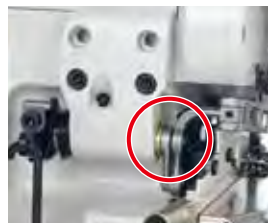
<Presser arm shaft at its upper position>
