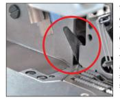
The cutter knife automatically descends to cut a tape and/or thread chain when the sensor detects the edge of the fabric. Since the length of tape or thread chain that remains after a cut can be adjusted by stitch counting as desired, no skilled operator is needed.
