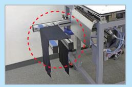
Equipped with a stacker (except the LSN-420 series), stacking the finished fabric is performed neatly and consistently.
