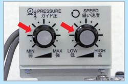
The machine speed and the edge controller pressure can be readily adjusted with the knobs placed at the front of the machine.
