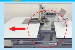
The sewing machine table slides smoothly, so threading the machine, maintenance and cleaning around the machine are easy.
