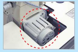
Equipped with a direct drive motor, the machine has a very good response when it starts/stops, and the underside of the machine table is clear.
