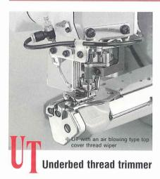
Eliminates the tedious job of trimming the needle and looper threads. All you have to do is press the treadle with your heel, thus increasing machine efficiency. Two types, electric and pneumatic, are available. (An air blowing type top cover thread wiper is optional for the UT with a top cover thread wiper.)
