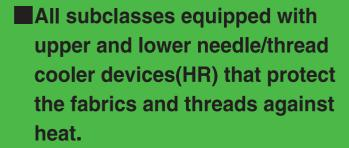
Heat is generated on the needle due to friction when the needle penetrates the fabric at high speeds. This causes thread breakage and/or stitch skipping. This series is equipped with HR device that always prevents heat generation on the point of the needle, allowing the thread to move smoothly and producing the stitches uniformly.
