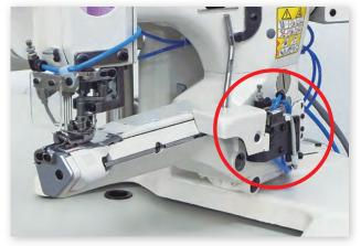
Threads are easily cut, by pressing the treadle with heel. This feature greatly enhances operator efficiency and allows for increased production. (Except for FW204S series)
