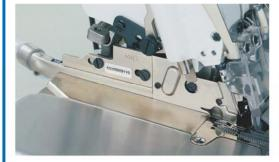
The suction inlet is positioned vertical to the needle plate and on the side of the needle (s) .
