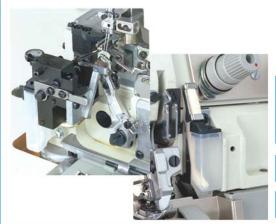
This device reliably reduces heat generated at the point of the needle by friction when they penetrate the fabric with the machine running at high speed. In addition, it allows the thread to move smoothly through the machine, decreasing the cause of stitch skipping and/or thread breakage. As a result, the machine produces uniform stitches.
