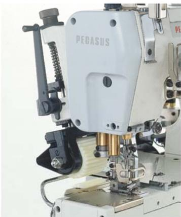
The roller pulls the fabric from behind the needle drop hole. Thanks to this device, the machine smoothly sews difficult-to-feed fabrics, providing beautifully finished products with no plyshifting.
