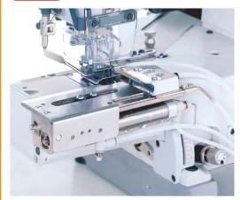
This sliding type hemming guide folds the fabric to form a hem in hemming operations. Thanks to this device, hemming is easy and resulting hem width is uniform, so quality products are obtained. Two types of driving sources are available, pneumatic and electric.
