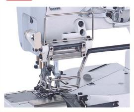
The elastic lace feeder with a mechanical metering device (MD), feeds the elastic lace according to the feeding amount of fabric that is fed, so that the feed of the elastic lace is even if the machine speed is changed. This results in uniform and beautiful elastic lace attaching operations.
